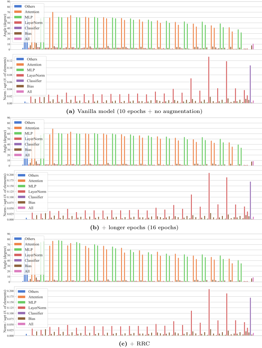
Fig. J: Layer-wise angle and norm across different augmentations. Displayed from top to bottom are the angle and norm for the vanilla model (10 epochs + no augmentation), +longer epochs (16 epochs), and +RRC. Each augmentation is applied incrementally. These metrics demonstrate consistency regardless of the augmentations from left (first layer) to right (last layer).
